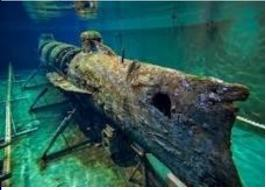
The Hunley is now in a 75,000-gallon tank filled with sodium hydroxide solution designed to leach out the salts threatening the submarine. The solution is mainly to loosen up the rock-like- layer of sand, sediment, and rust. All of the 8-man crew members remains where respectfully removed and were given a proper confederate burial.
